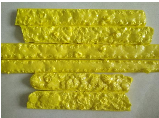
Figure 2.5. Photograph of synthesized AgGaS 2 polycrystal by two temperature vapor transport method [11].
